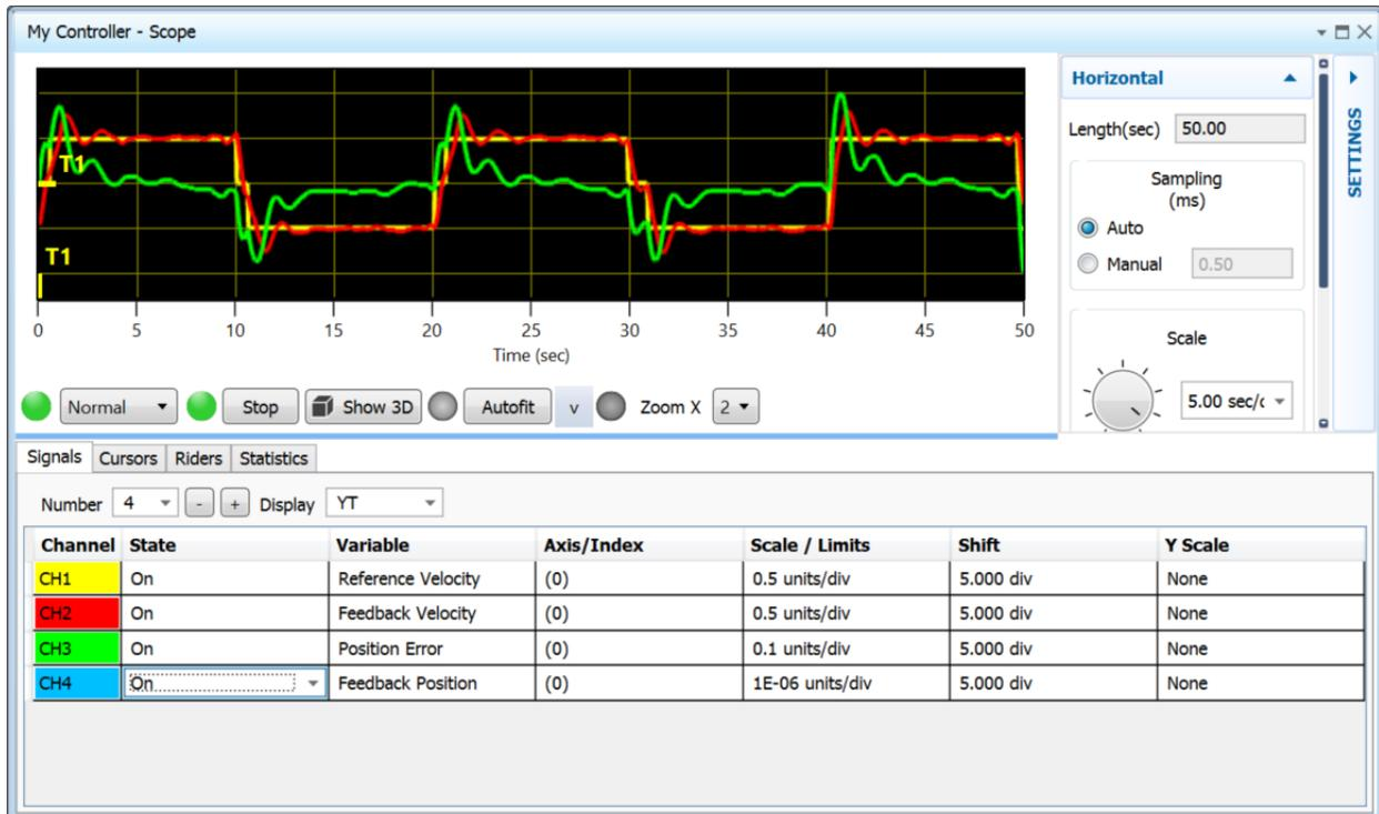
Figure 73: MMI Studio’s scope output giving validity to tuning parameters during a Motion Manager back and forth move. Feedback velocity follows reference velocity and a low, steady-state position error. Note the scale of the position error is 0.1 units/division.
